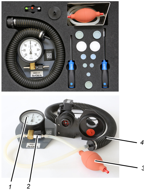
Fig. 4 Testing of the Control Valves
